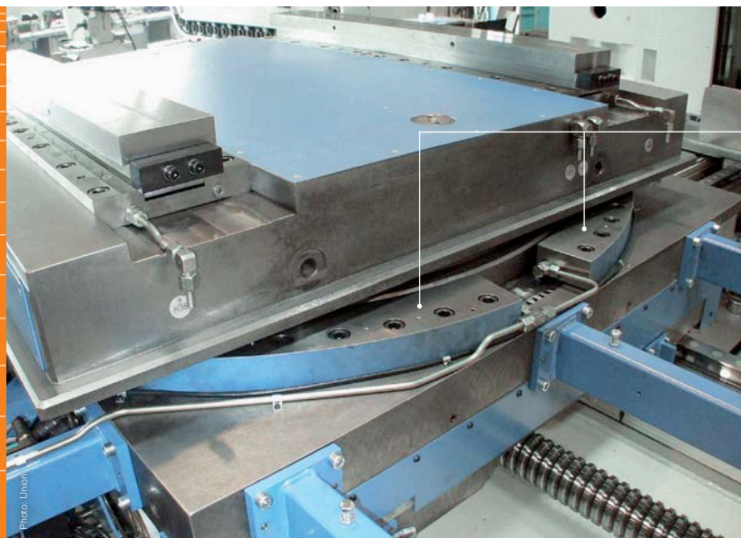
Segmented clamping cassettes with KOSTYRKA® clamping discs form an annular table clamp here.
