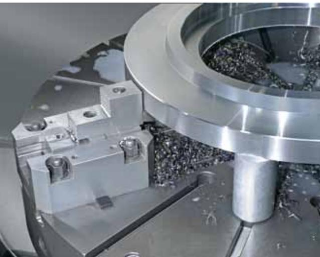
For holding workpieces in milling and turning centres, HILMA box jaws are the first choice. This new development combines a number of striking advantages compared with the normal level of technology available in the market.
